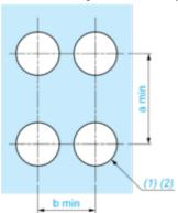
(1) Diameter on finished panel or support (2) Ø22.5 mm recommended (Ø22.3  $_0^{+0.4}$ ) / Ø0.89 in. recommended (Ø0.88 in.  $_0^{+0.016}$ )
